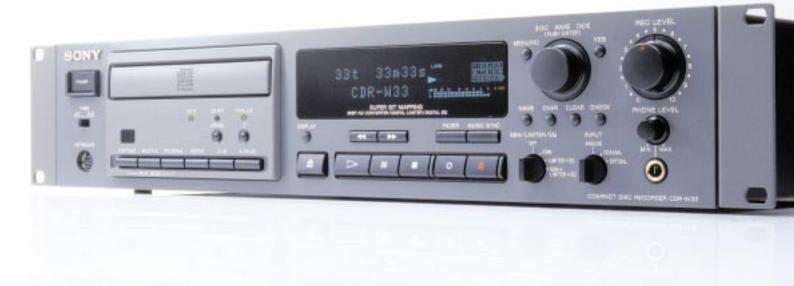
The Sony CDR-W33 is a compact disc recorder developed with the achievement of outstanding sound quality as a central design objective. Through the use of Super Bit Mapping recording technology and 24-bit A to D and D to A conversion, the CDR-W33 meets this target and is able to achieve high sound quality approaching that of 20-bit recording quality.
