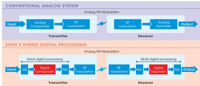
DSP optimizes the audio signal processing applied between the transmitter and receiver. It provides superb transient response performance. While analog companding systems cannot reproduce sounds such as a bell or tee shot with precision, Sony's Hybrid Digital Processing can reproduce them very accurately.
