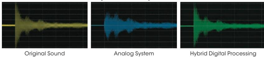
DSP also can correct characteristics of frequency response in the transmission process for precise reproduction of original sounds.
