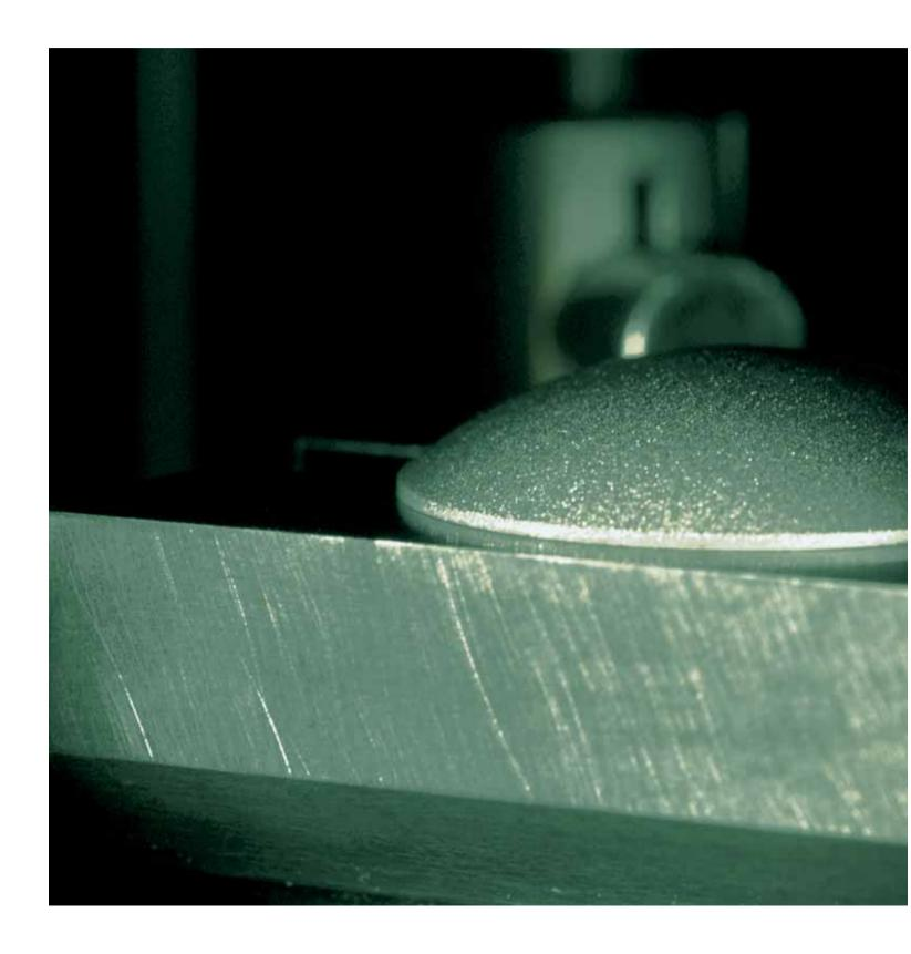
Thanks to recently developed industrial processes, diamond can now be synthesised reliably in significant quantities, and in a variety of forms. It is a miracle material. Resistant to chemical attack, transparent to ultra-violet and infrared, an exceptional heat conductor and electrical insulator, its applications are growing fast. But the properties most commonly exploited – and which B&W has used to dazzling effect – are its remarkable strength and stiffness.
