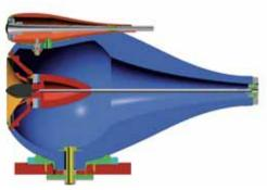
Dream weaving Waves and squares generally don't mix. Which is one reason why you'll find so few straight lines on an 800 Series speaker. But there is one component where square makes sense. The kind of homogeneous materials used to make conventional midrange driver cones are prone to the development of unwanted concentric standing waves.
