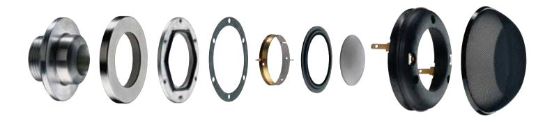
The tube-loaded tweeter that crowned speakers in the Nautilus 800 Series was a development of that pioneered by B&W's revolutionary Nautilus™ speaker. The concept hasn't changed a bit, but inside we've introduced a number of important refinements. First, there is the alternative on some 800 Series models of our ultimate tweeter dome formed of synthetic diamond, which gets even closer to ideal tweeter behaviour than previously possible, within and above the audible range.
