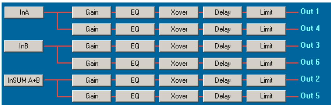
In the stereo modes, you can choose whether the Stereo Link should be activated or not. In Mono Mode, this option is not available.
