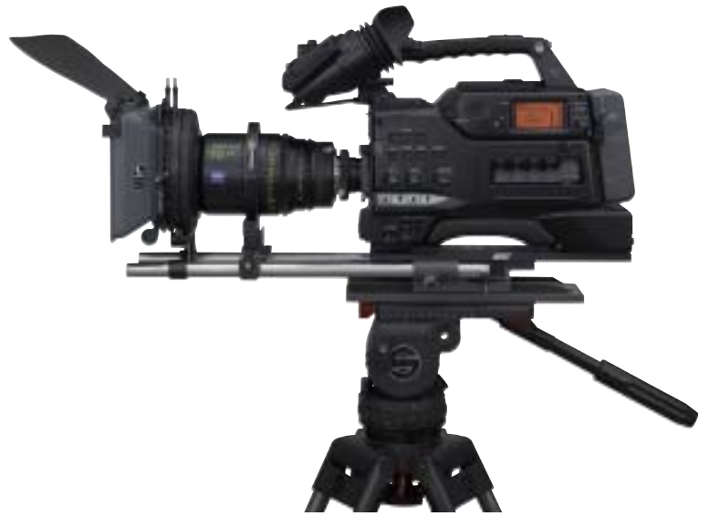
Cinema lens on HVR-S270E with an adaptor
