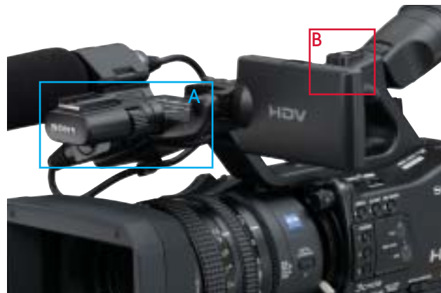
A:Removable Front Shoe B:Screw Hole
