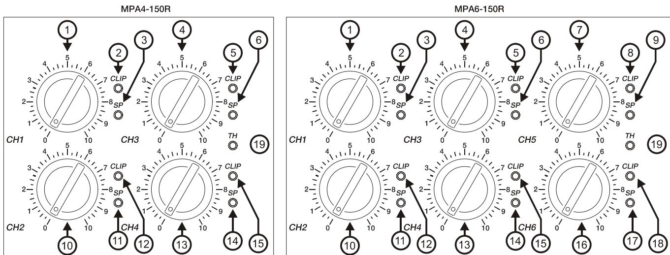
These attenuators allow the connection of different mixers, an independent volume control and the connection of speakers not able to handle the amplifiers maximum output power, thus avoiding the risk of damaging them with the mixers or preamps volume control.
