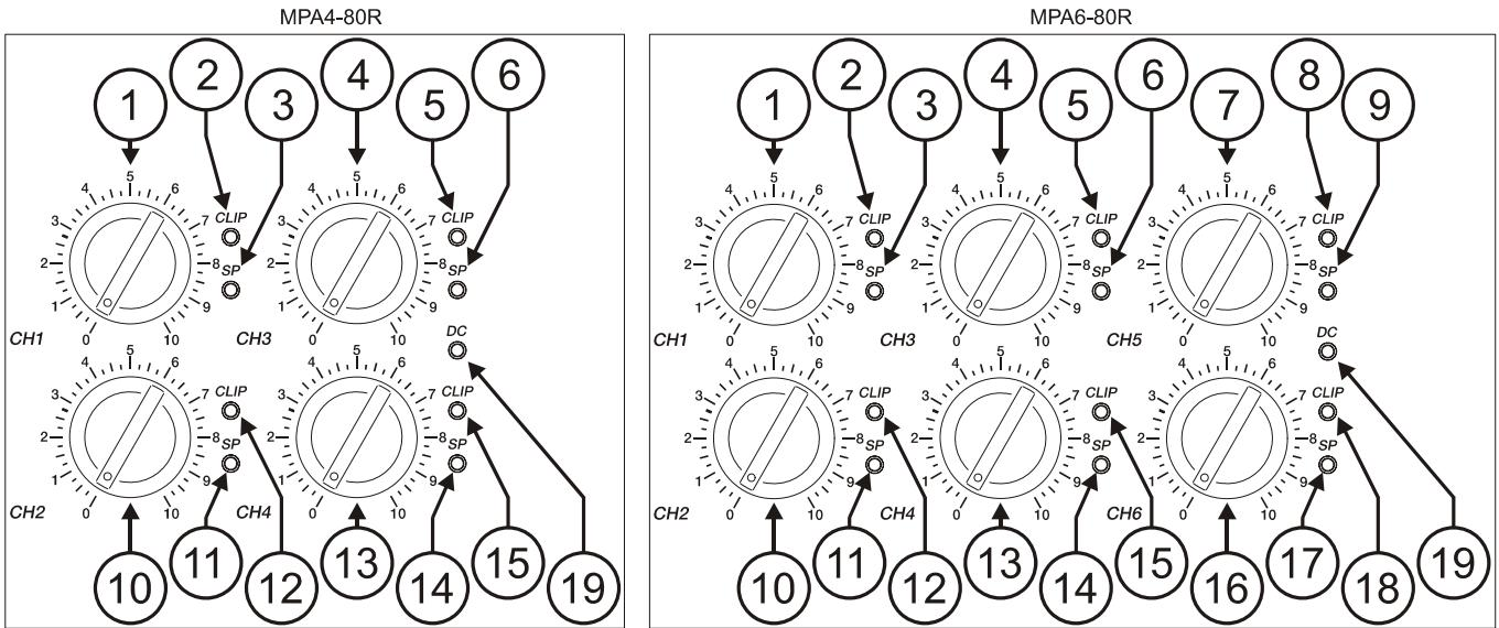
These attenuators allow the connection of different mixers, an independent volume control and the connection of speakers not able to handle the amplifiers maximum output power, thus avoiding the risk of damaging them with the mixers or preamps volume control.
