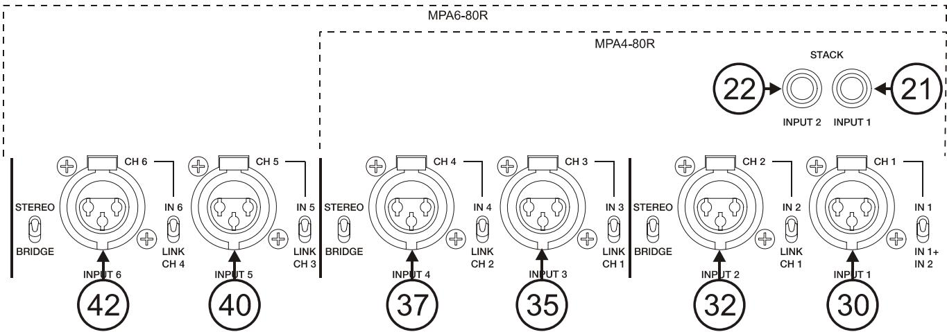
The signal input connections (30, 32, 35, 37, 40, 42) are electronically balanced XLR-3 sockets, with input impedance higher than  $20\text{k}\Omega$  and a nominal sensitivity of  $0\text{dBV}(1\text{V})$ . Pin assignment:
