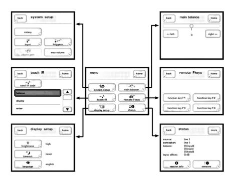
Pressing the front panel **Menu** button to the left of the LCD touchscreen brings up a comprehensive *main menu system*, the top two levels of which are shown above. This menu system provides access to many installation-specific features that let you customize how the CAP-2100 works within the context of your particular system.
