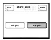
The phono gain menu is only active if the optional **phono module** is installed; otherwise it is grayed out. When it is installed, the CAP-2100 will automatically recognize it, rename the **line 1** input to **phono**, and activate the input on the main menu.
