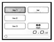
The **operational menu** provides easy access to the most basic functions of the integrated amplifier: **input selection** and **tape monitor**. It also provides both a numeric and a graphic depiction of the current volume setting
