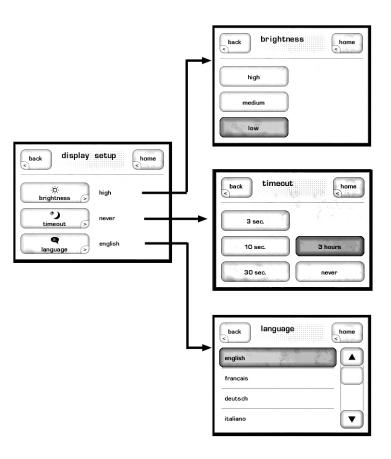
This button brings up the **display setup** menu. It allows you to configure the CAP-2100's LCD screen *brightness*, the display *timeout*, and the *language* used in the touchscreen and menu system.
