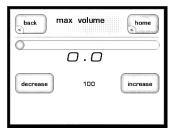
The **max volume** screen allows you to establish a maximum volume setting for your system. This scale runs from 0 to 100, with 100 indicating that you do not want any artificial limit placed on the maximum gain your integrated amplifier can provide.
