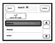
The CAP-2100 provides discrete infrared (IR) command codes for all its functions, a list that extends far beyond what is required by normal remote controls. However, many of these functions are critical if you plan to create a customized remote control with macros that take command of your entire system. Without these discrete codes, many of the macros you might want to create will simply not work reliably.
