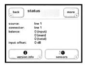
The primary function of the **status** screen is to provide information about the current operating status of the CAP-2100. It also provides access to *version info* screen, which displays information about the unit's software, and the *sensors* screen, which displays information from the internal sensors about the temperature and input power.
