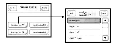
The remote control supplied with the CAP-2100 has four **function keys** (**Fkeys**) that allow you to have instant, easy access to specific system functions that might otherwise be buried in a menu somewhere.
