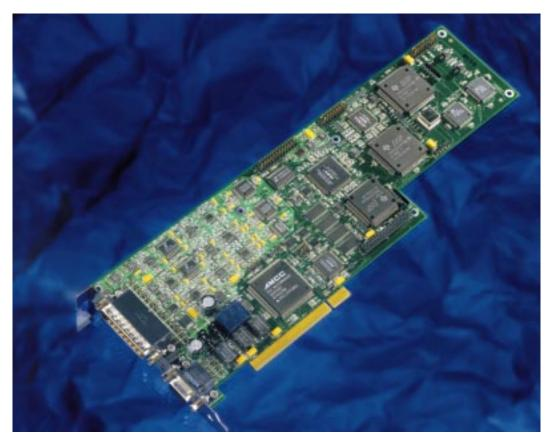
6 STEREO MPEG DEVICES SIMULTANEOUS PRODUCTION AND ON-AIR PLAYBACK THREE 32-BIT FLOATING POINT DSPS 20-BIT A/D AND D/A CONVERTERS
